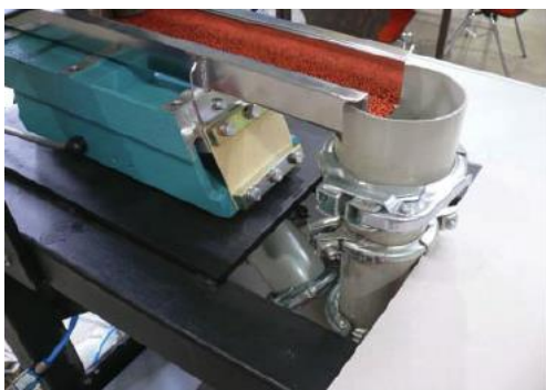
Fig. 5: The speed of the vibrating chute is controlled automatically.
