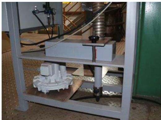
Fig. 2: The radial blower draws the dust-laden air through the photometer.
