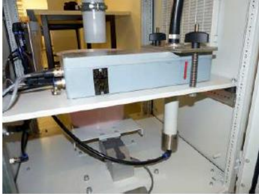
Fig. 2: The dust particles are drawn by vacuum through the photometer.
